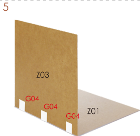
Use G04 to fix the junction of two pieces of plexiglass. (use transparent tape to replace G04)
